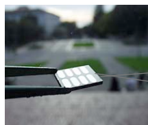
Nano solar cell: Inorganic nanorods embedded in semiconducting polymer, sandwiched between two electrodes
