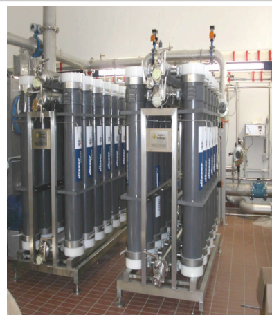
An ultrafiltration plant in Jachenhausen, Germany
