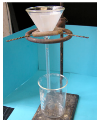
Figure 1. Funnel supported by ring with beaker underneath to catch effluent [1].
