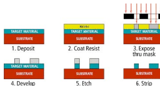
Figure 10. Photolithography, a process of chiseling away material to make integrated circuits [13].
